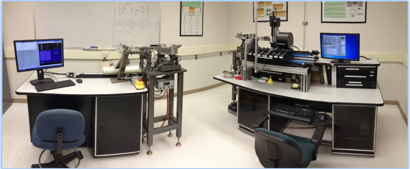
Figure 34. New PIT Tag Sorter automation (left) and the Automated PIT Tag Testing System (APTTS) automation (right).
